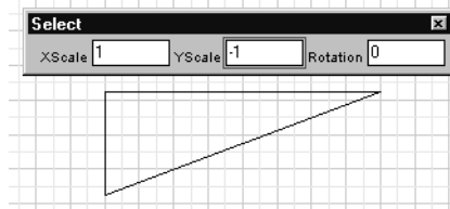
Using a value of -1 in the Y Scale field to flip the triangle
